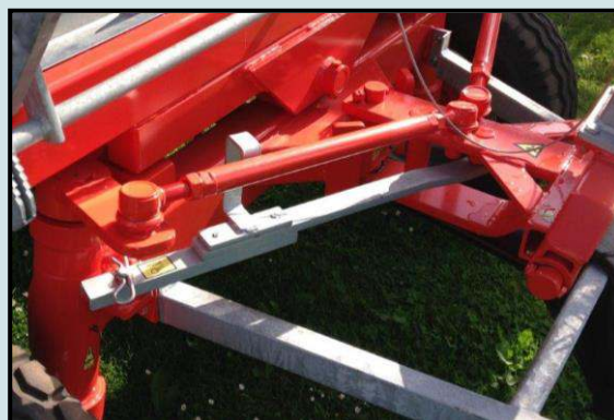
Manual control with locking pawl mounted
